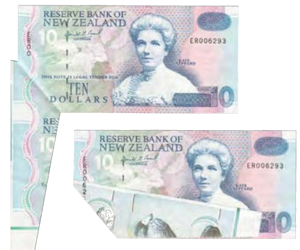
This error was caused by a fold in the paper, after the banknote sheets were printed but before the serial numbers were printed and the sheets guillotined. This creates a "flap."
